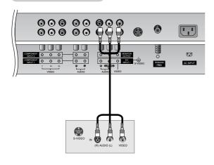
The TV has a special signal output capability which allows you to hook up a second TV or monitor.
